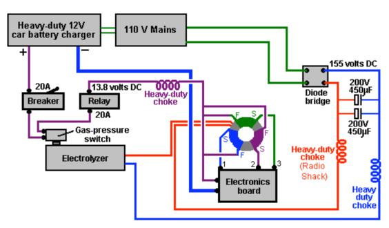
Here, instead of an inverter to create 110 volts AC, a car battery charger or mains Power Supply Unit is needed to provide the same voltage that the vehicle electrics would have provided. It would probably be worth putting a large value capacitor across the output of
