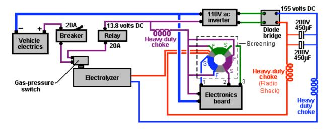
It is important to include heavy-duty chokes (coils) in both sides of the high voltage power supply and in the 13.8 volt positive lead coming from the vehicle electrics. These choke formers are available from Radio Shack in the USA, through it is perfectly ok to wind these chokes on laminated iron pieces taken from an old mains power transformer frame.
