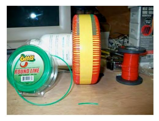
As you can see here, Bob uses short lengths of plastic strimmer cable as spacers for the outside of the toroid, though the picture above has been taken to show what a partially prepared secondary winding looks like when its windings are being moved into very accurate positions.
