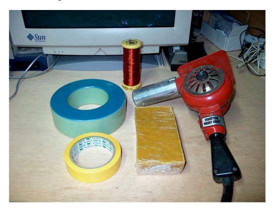
Of paramount importance with the toroid is that unlike traditional transformer design, the secondary is wound first, and the windings must be evenly spaced where they fan out from the center of the core. This means even though they are tightly packed right up against one another at the center hole, they must not be wound so that they bunch up
