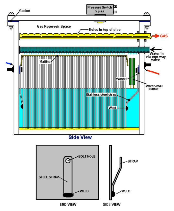
To combat splashing of the electrolyte, a layer of aquarium matting is placed over the tops of the plates. In the diagram above, only a few of the 101 plates are shown, in order to keep the drawing narrow enough to fit on the page. The plates at each end have a stainless steel strap welded to them in order to allow for simple and robust electrical connections to be made through the case.
