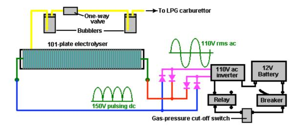
As mains voltage is quoted as an average figure ("root-mean-square") it has a peak voltage of 41% more than that. This means that the pulsing DC has a voltage peak of just over 150 volts for the nominal 110 volt AC output from the inverter.
