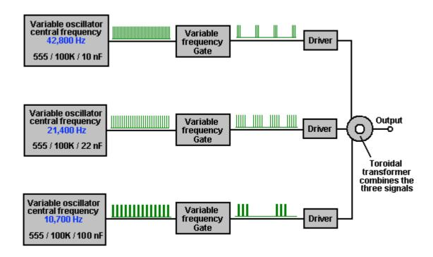
In Bob's electrolyser build, those frequencies were about 42.8 KHz, 21.4 KHz and 10.7 KHz but please don't get the wrong impression here, there is no single exact frequency
