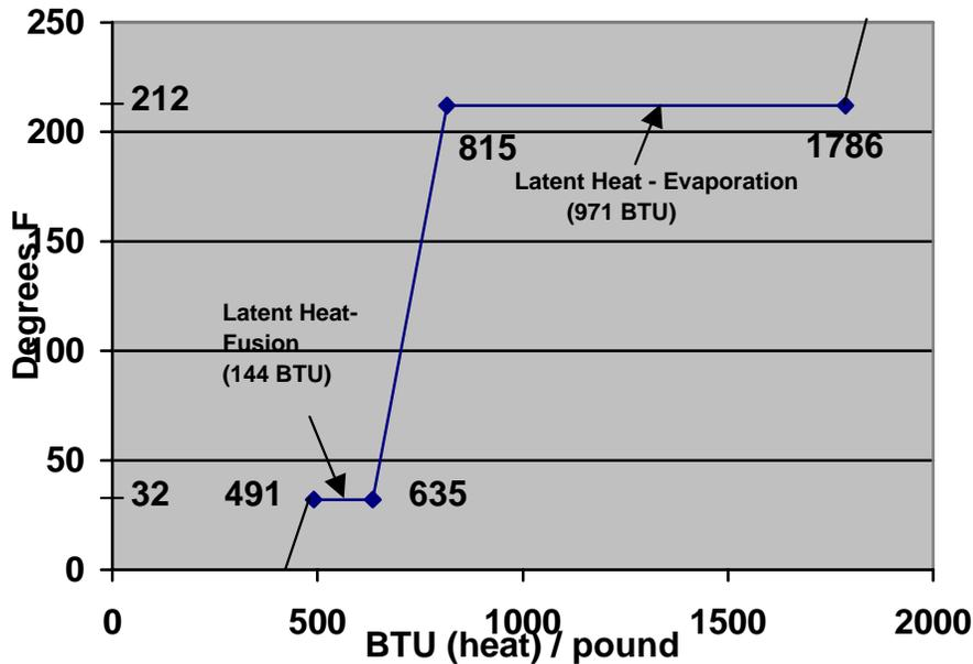
In the above graph, the amount of heat added to water is referenced from 0° Kelvin (absolute zero). The latent heat of fusion of water is 144 BTU per pound. In the process of freezing, water releases the same amount of heat (144 BTU / pound) that is absorbed in the process of melting.
