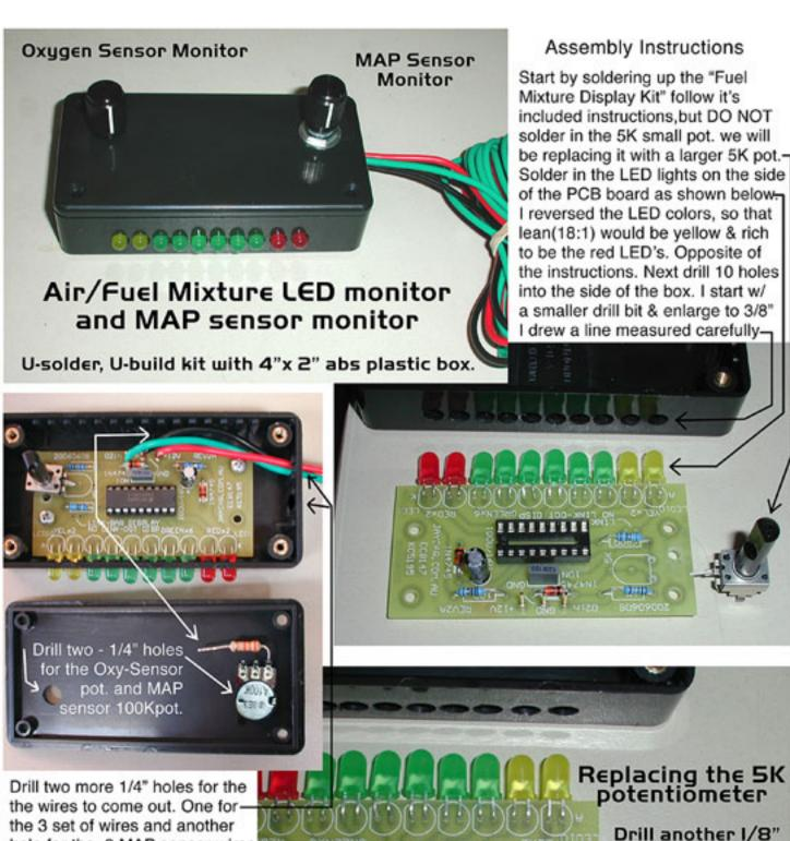
Drill two more 1/4" holes for the the wires to come out. One for the 3 set of wires and another hole for the 2 MAP sensor wires. Solder on the 33k resistor to one outside leg of the 50K pot. The paired speaker wires get soldered to the other 2 legs. The resistor gets grounded to the black wire on the FMD PCB board terminal. The black wire is ground, I solder on a 2" long wire to connect the pot to the (-) terminal post. I used 2' of black wire off the end of the wires that came with the kit.
