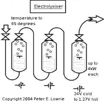
Ametered supply of hot <sup>14</sup> engine exhaust gas is intoduced to the bottom of a stainless steel pressure vessel. The gas percolates through four electrodes knocking off some gas bubbles on it's way up through the electrolyte. The gas output from cell 1 is repeated in cells 2 and 3 which helps to provide a *richer* concentration of gas called electrolytic Gas. This is a fuel gas.
