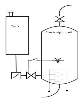
The tank contains distilled water – the electrolyte is maintained within the cells. Because KOH does not dissipate into the gas flow the concentration is maintained within for a considerable time.
