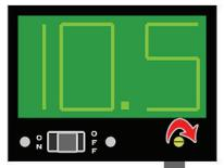
CURRENT LIMIT POT CLOCKWISE DECREASES AMPS AIR BOX FITTING CAN BE INSTALLED IN THE AIR BOX OR AIR DUCT THAT GOES TO THE THROTTLE BODY. SOME VEHICLES RESPOND BETTER BEFORE THE MAP/MAP SENSOR AND SOME AFTER.
