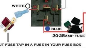
PUT FUSE TAP IN A FUSE IN YOUR FUSE BOX THAT HAS POWER ONLY WHEN THE ENGINE IS RUNNING THEN CONNECT TO 86 OF RELAY.
