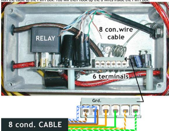
Above is the inside of the PWM, you need to connect the 8 wires to the 6 terminals and one to ground to the grounded case. One wire to power+
