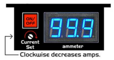
To increase amps adjust the tiny screw on the display. It takes a tiny jeweler's screwdriver to do the trick. The amps are factory set at 10 amps. For the 77 cell, and 20 amps for the 14/7 cell.
