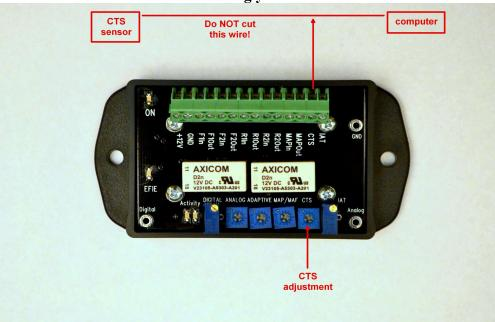
Locate your **CTS. A word of caution:** Some vehicles have 2 almost identical **CTS**. (coolant temperature sensor's) One is for operation of a temperature gauge or indicator, and one that
