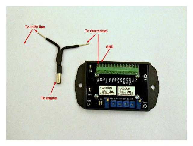
With the new Tstat switching device, you will need to solder on lengths of wire to the Tstat stub wires in sufficient length to reach your 12 v ignition switched power source and to reach the 12v input of your Tuning 101 Automated AFR Control Center. Refer to above photo. Connect your terminal marked GND to either the negative terminal of the battery or a GOOD clean chassis ground.
