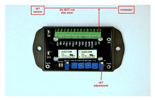
Locate your IAT (intake air temperature) sensor. There will be 2 wires going to the sensor. You will **NOT** be cutting any wires. You will skin off some of the insulation from the signal wire. Refer to your manuals diagram. Or you can refer to the document Identifying your signal wires. Solder on a length of wire sufficient in length to reach your AFR Control Center and attach it in the terminal marked IAT as pictured above.
